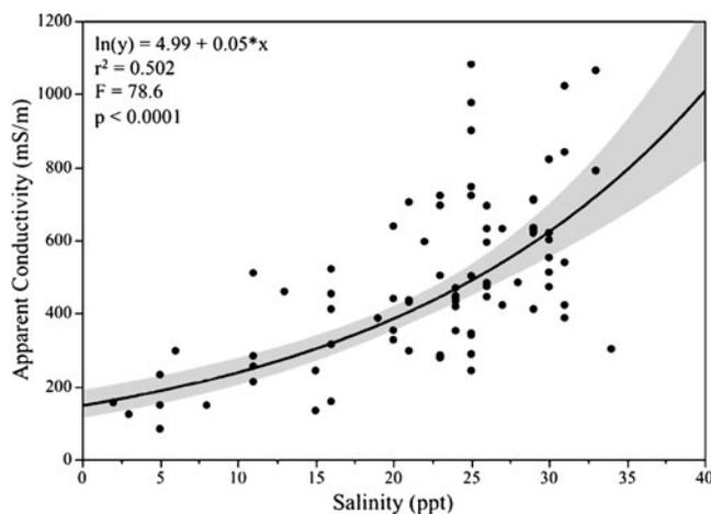
**Fig. 3** Regression of apparent conductivity ( $EC_a$ ) and pore water salinity.  $EC_a$  was measured at 50 cm above the marsh surface, whereas salinity was directly measured with a sipper and refractometer. The shaded region represents 95% confidence interval of the regression line
