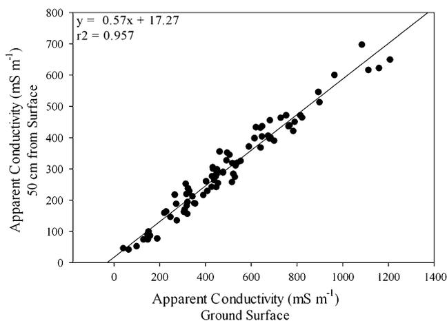
**Fig. 2** Comparison of apparent conductivity ( $EC_a$ ) at different sampling heights (0 and 50 cm) above marsh surface
