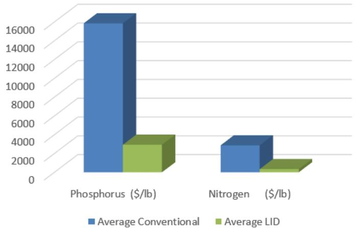
Cost comparison by Scott Horsley, Horsley Witten Group, Inc. based on comparison between a conventional detention basin vs. gravel wetland and bioretention. See supplemental information online for more details on how this was calculated.
